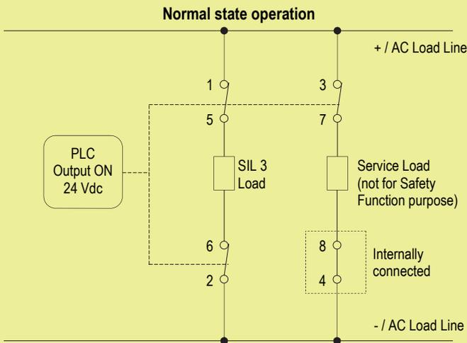
**Contacts 1-5 and 2-6:** in normal operation the relay is energized, contacts are closed, SIL 3 load is energized.
