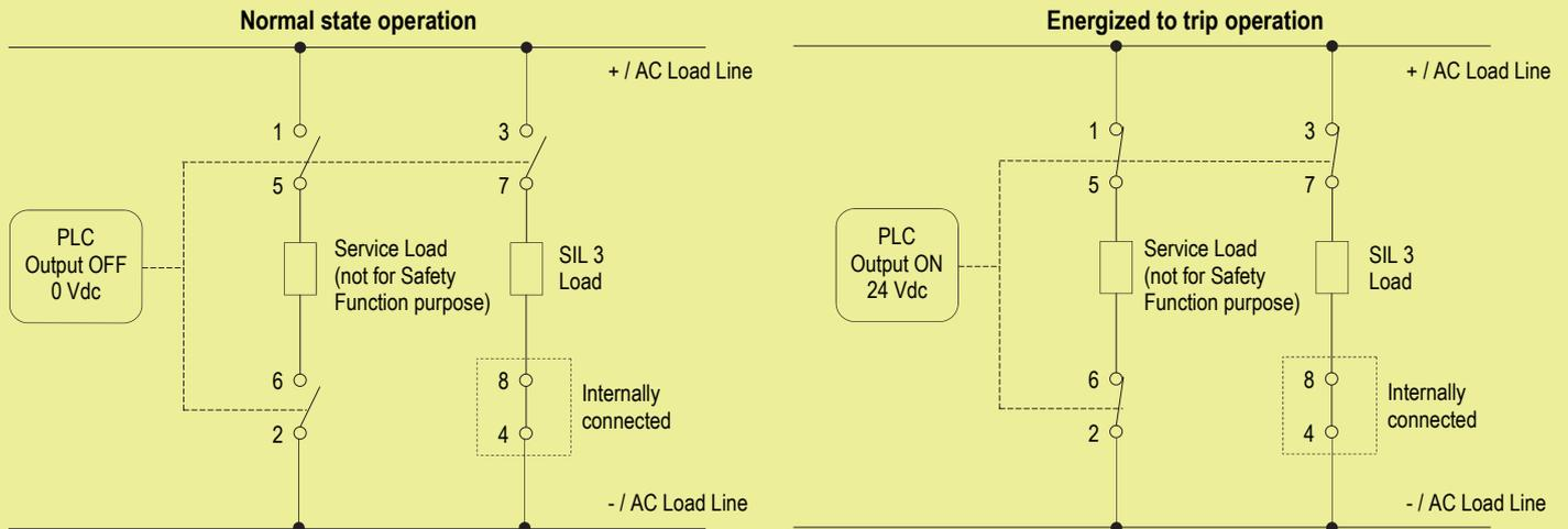
**Contacts 1-5 and 2-6:** in normal operation the relay is de-energized, contacts are open, Service Load load (not for Safety Function purpose) is de-energized.
