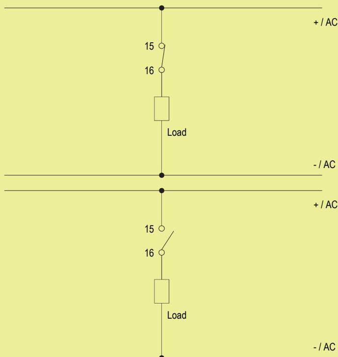
**Contacts 15-16:** Voltage free contact for Line and Load Fault detection. Can be connected in series with other relay units for common monitoring. Normally closed when there is not Fault condition.
