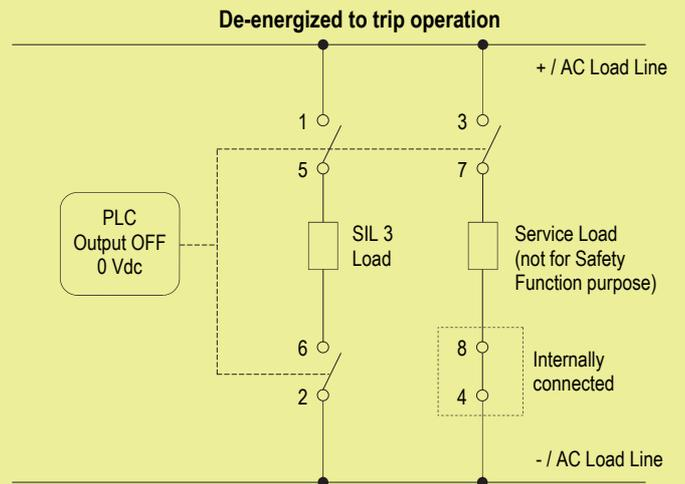
**Contacts 1-5 and 2-6:** the SIL 3 Safety Function is met when the relay is de-energized, contacts are open, SIL 3 load is de-energized.
