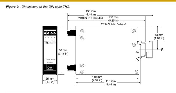
Figure 10. Dimensions of the THZ HPP unit.
