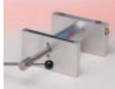
The screw pump is designed for very easy tabletop operation and offers exceptional pressure control. Generates up to 350 bar / 5,000 psi. Medium is water or oil.
