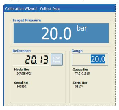
During a calibration, the Target Pressure is the next profile value and the Reference and Gauge pressures are indicated below. The Gauge value is, by default, the same value as the Target Pressure. However, the value can be changed by the user to match what is read from the gauge.
