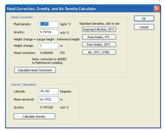
The calculator uses Fluid density, Gravity and Height change to calculate a correction that is added to the pressure measured by the reference.
