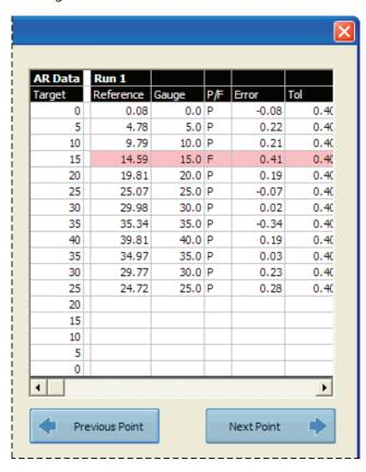
As the calibration progresses, the gauge will pass or fail at each profile point, or Target Pressure. To pass, the Gauge must be equivalent to the Reference within the tolerance range. The tolerance is defined as the accuracy of the gauge at the measured pressure. The data are displayed in a box at the right of the calibration window.
