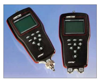
JOFRA HPC500 calibrators feature deadweight tester accuracy in a modern digital package. The HPC is available as an independent calibrator or in one of 6 ready-for-test systems that are complete and equipped to meet any need for pressure calibration.
